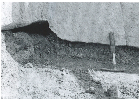
Plate 2 Discontinuity in Grade III granite, infilled with alluvial sand
