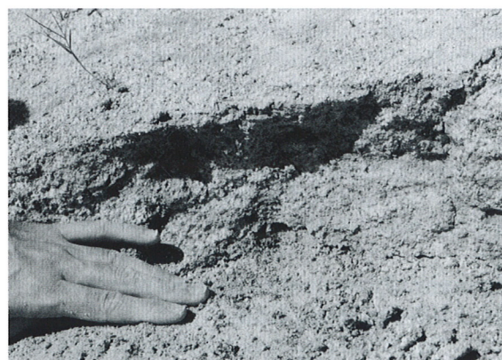
Plate 1 Discontinuity with thin (<1mm) clay infill in Grade V granite
